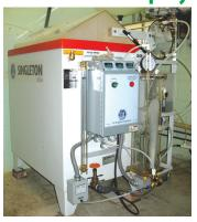
Raytec Screws are tested in a salt spray chamber in accordance with American Society for Testing and Materials- ASTM B117 standards.
