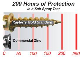
Hours of Red Rust Protection Actual hours of rust protection depend on many factors such as geographical location. **Commercial Zinc Screw**
